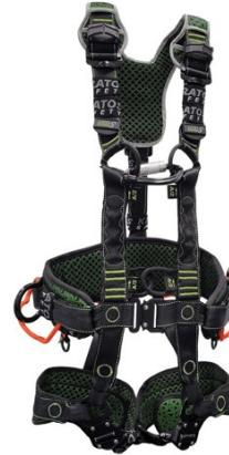
Attachment points - 1 textile sternal attachment point (A) and 1 dorsal attachment point (A) for fall arrest, a dorsal attachment loop (A) for double retractable fall arresters, 1 ventral attachment point for connecting the fall arrest carriage of a cable or rail system. 2 lateral D-rings for work positioning.
